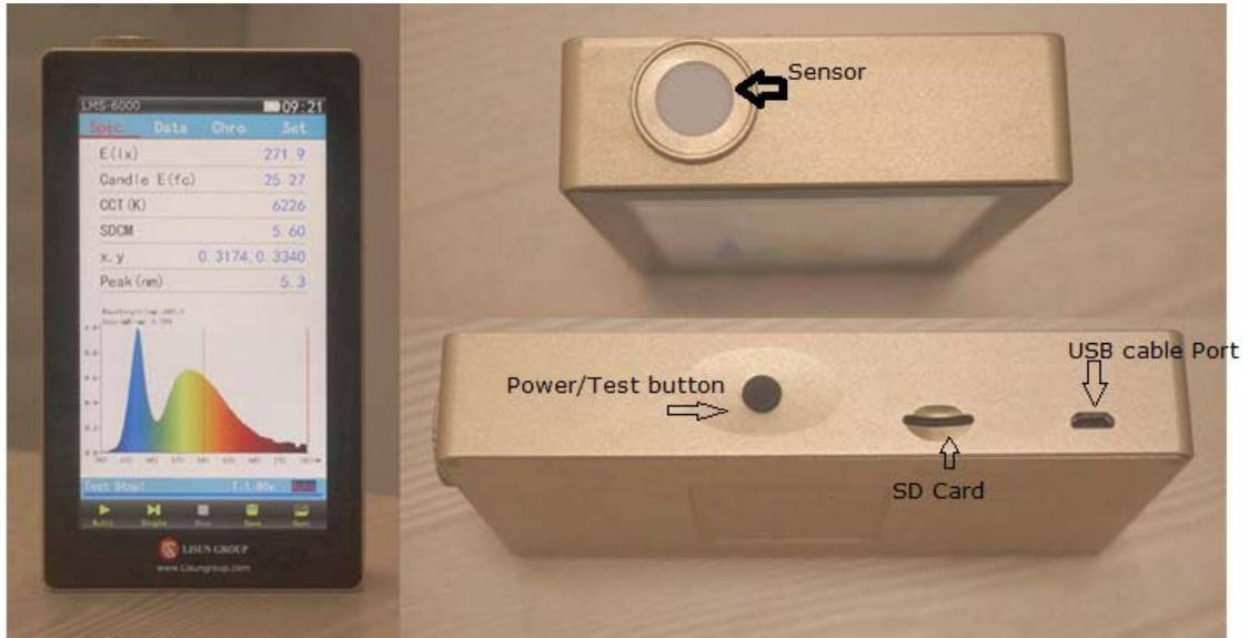
You need to hold the LMS-6000 and let the Milky piece sensor towards to the light source, keep about **5 seconds** if do single test, then you will get the accuracy test results.
